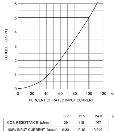
**CHARACTERISTICS** - With no electrical excitation, the shaft freely rotates. With electrical excitation, the shaft becomes coupled to the housing. Torque is proportional to input current (see torque graph), and independent of RPM. While the load torque is less than the output torque, the shaft won't rotate. When the load torque is increased, the brake will slip smoothly at the torque level set by the coil input current.
