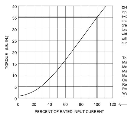
CHARACTERISTICS - With no electrical excitation, the input shaft & output shaft freely rotate. With electrical excitation, the input shaft becomes coupled to the output shaft. Torque is proportional to input current (see torque graph), and independent of slip RPM. While the load torque is less than the output torque, the clutch drives without slip. When the load torque is increased, the clutch will slip smoothly at the torque level set by the coil input current.
