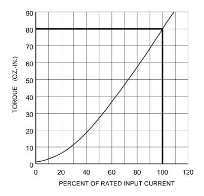
CHARACTERISTICS - With no electrical excitation, the input and output shafts freely rotate. With electrical excitation, the input shaft becomes coupled to the output shaft. Torque is proportional to input current (see torque graph), and independent of RPM. While the load torque is less than the output torque, the input shaft and output shaft are locked together. When the load torque is increased, the clutch will slip smoothly at the torque level set by the coil input current.
