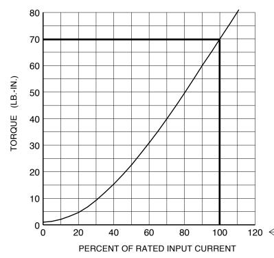
CHARACTERISTICS - With no electrical excitation, the input shaft & output shaft freely rotate. With electrical excitation, the input shaft becomes coupled to the output shaft. Torque is proportional to input current (see torque graph), and independent of slip RPM. While the load torque is less than the output torque, the clutch drives without slip. When the load torque is increased, the clutch will slip smoothly at the torque level set by the coil input current.
